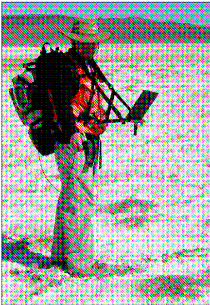
Figure 5: Kratt using an Analytical Spectral Devices field spectrometer (ASD) to check remote sensing data results
