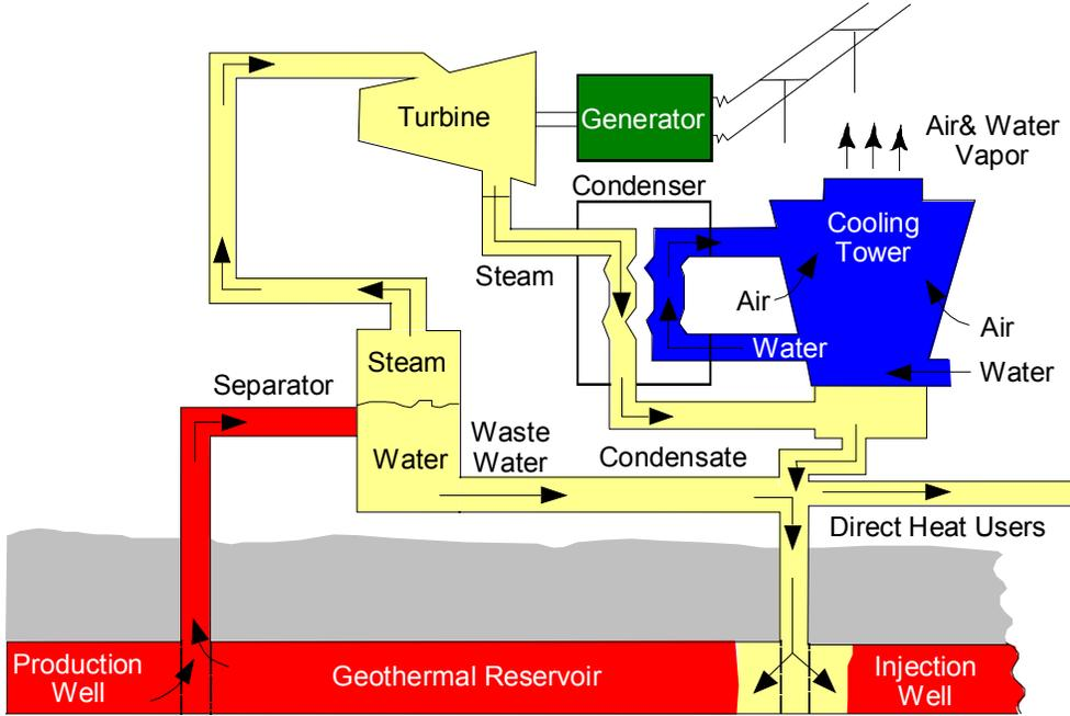
**Figure 28: Double Flash Steam Power Plant Schematic**
