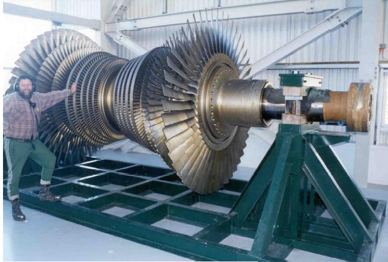
**Figure 53: Turbine Blade at Lardarello, Italy Geothermal Facility**
