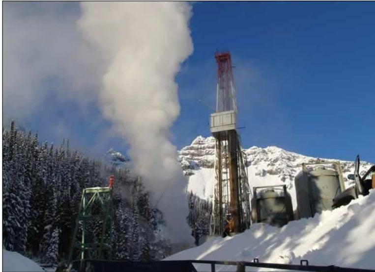
Flow test of well MC-6 at the South Meager geothermal project (Source: Western GeoPower)
