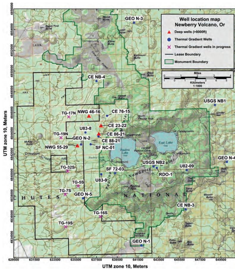
Figure 2. Well location map: Red triangles are deep exploration test wells; Davenport wells NWG 46-16 and NWG 55-29, California Energy wells CE 23-22 and CE 88-21. Blue dots are temperature gradient and shallow test wells. Red x are incomplete Davenport temperature gradient wells.
