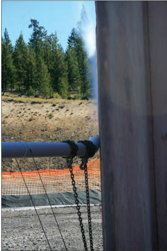
Figure 5. Initial gas flow from well NWG 46-16 through a 4-inch bleed line (8 September 2013).
