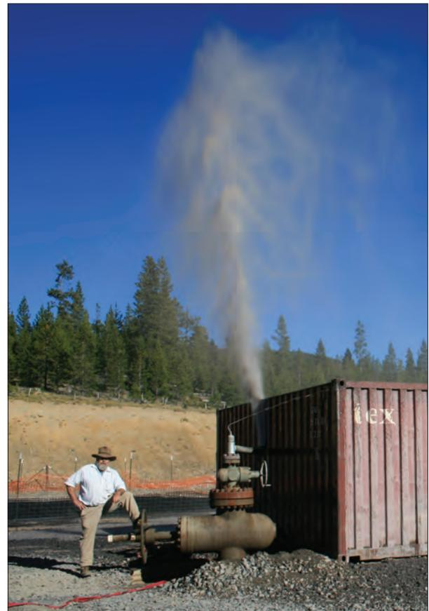
Figure 6. Author Al Weibel stands next to drilling fluid flowing through a 4-inch bleed line, approximately 45 minutes after the liquid flow commenced (8 September 2013). ■
