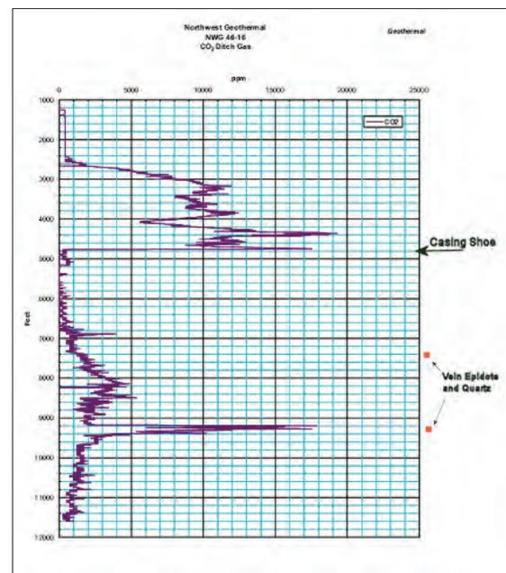
Figure 3. A graph showing CO<sub>2</sub> values measured by Epoch Mudlogging during drilling of well NWG 46-16. To the right are noted the depth of the casing shoe and the location of hydrothermally precipitated druze quartz and epidote observed in the drill cuttings. The shallow CO<sub>2</sub> shows are attributed to biogenic gas from organic matter within clastic layers.
