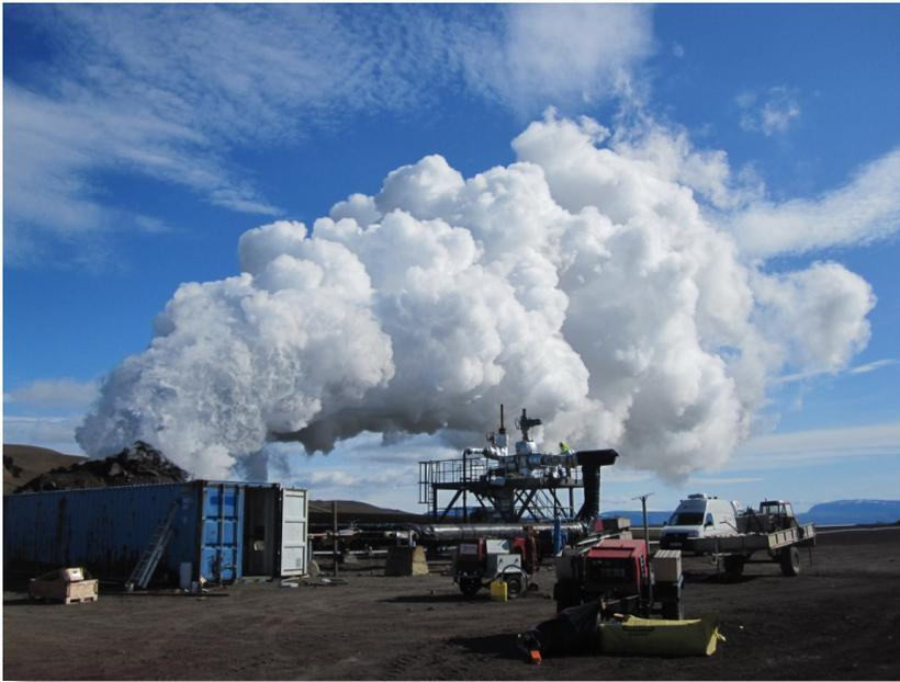
**Figure 1.** The flow of the well IDDP-1 into a rock muffler produced dry superheated 450°C steam with only 0.1-0.2% of non-condensable gases. Initially corrosion products gave the steam a dark color but after a few minutes it became clear and transparent. The condensate had a pH 2.5-3 due to its HCl content. However experiments on wet scrubbing to remove acid gases from the dry steam were very successful. (Photograph courtesy of Kristján Einarsson).
