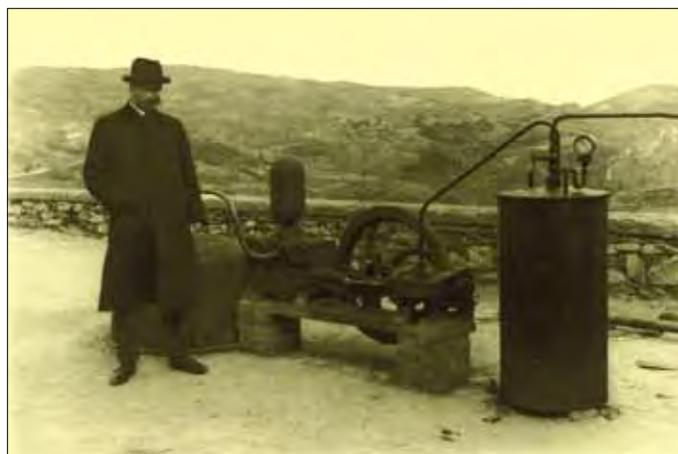
Photo of Prince Piero Ginori Conti at Larderello in 1904. He is standing by his invention, the first mechanical device to generate electricity from geothermal steam. COURTESY OF ENEL.
