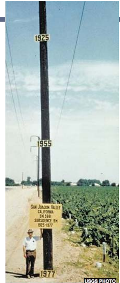
A pole is marked with the land levels in Mendota, California, showing the drastic sinking of the land for nearly a century.
